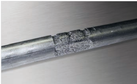
Crevice corrosion formed under a plastic clamp
